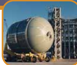
Aluminum Lithium Test Article (ALTA) Structural Test at the Cryostructural Test Facility
