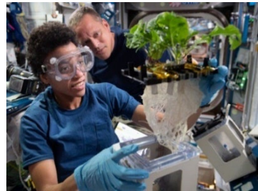
NASA astronauts Jessica Watkins and Bob Hines work on XROOTS, which uses liquid- and air-based techniques to grow plants rather than traditional growth media.
