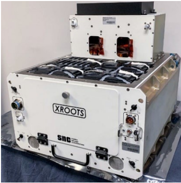
The eXposed Root On-Orbit Test System (XROOTS) grows plants in the microgravity environment of the ISS and evaluates nutrient delivery and recovery techniques such as aeroponics over the course of a full plant growth cycle. (Source: NASA)
