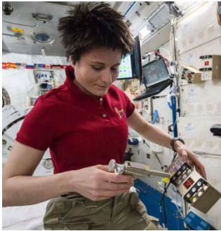
ESA Astronaut Samantha Cristoforetti activates all four BRIC-21 experiment canisters by injecting the growth medium to the samples. (Source: NASA)
