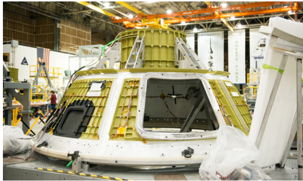
Eleven Nevada suppliers contributed to NASA's Artemis program. An example of the state's contributions is composite materials used for panels on Orion for Artemis I.
