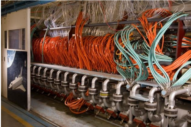
The segmented arc heater in the IHF.
