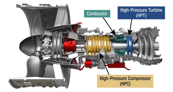
Cross-section of a turbofan jet engine showing the components of the HyTEC project's smaller engine core, with the compressor, combustor, and turbine noted. By shrinking the engine core, better fuel efficiency can be achieved. *Credits: NASA*
