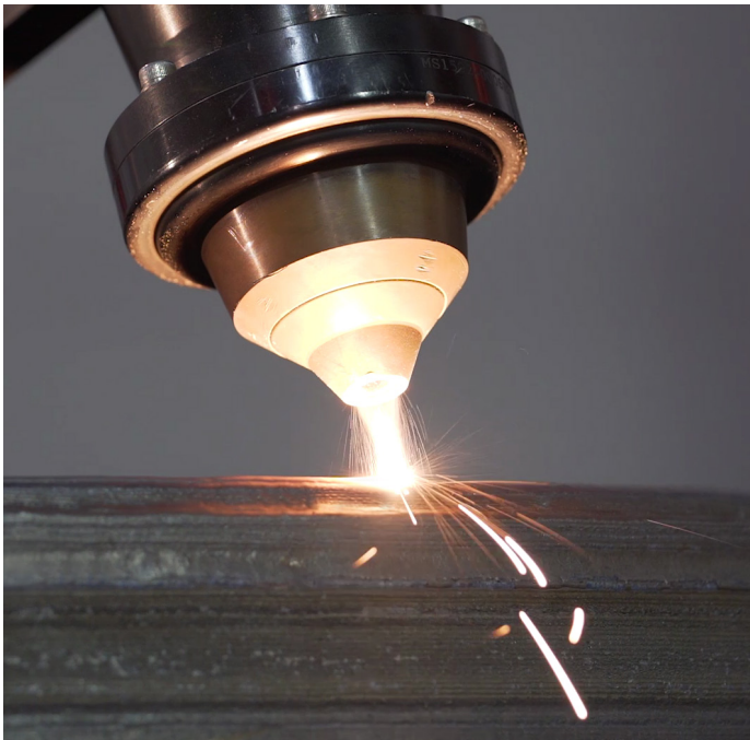
A laser powder directed energy deposition nozzle head building layers of JBK-75 alloy. Engineers and technologists at Marshall lead metal additive manufacturing, or 3D printing, developments for propulsion applications to mature processes. (NASA)
