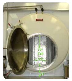
Sunspot is a 12-foot thermal vacuum facility located at the NASA Marshall Space Flight Center Environmental Test Facility (ETF) in Huntsville, AL.
