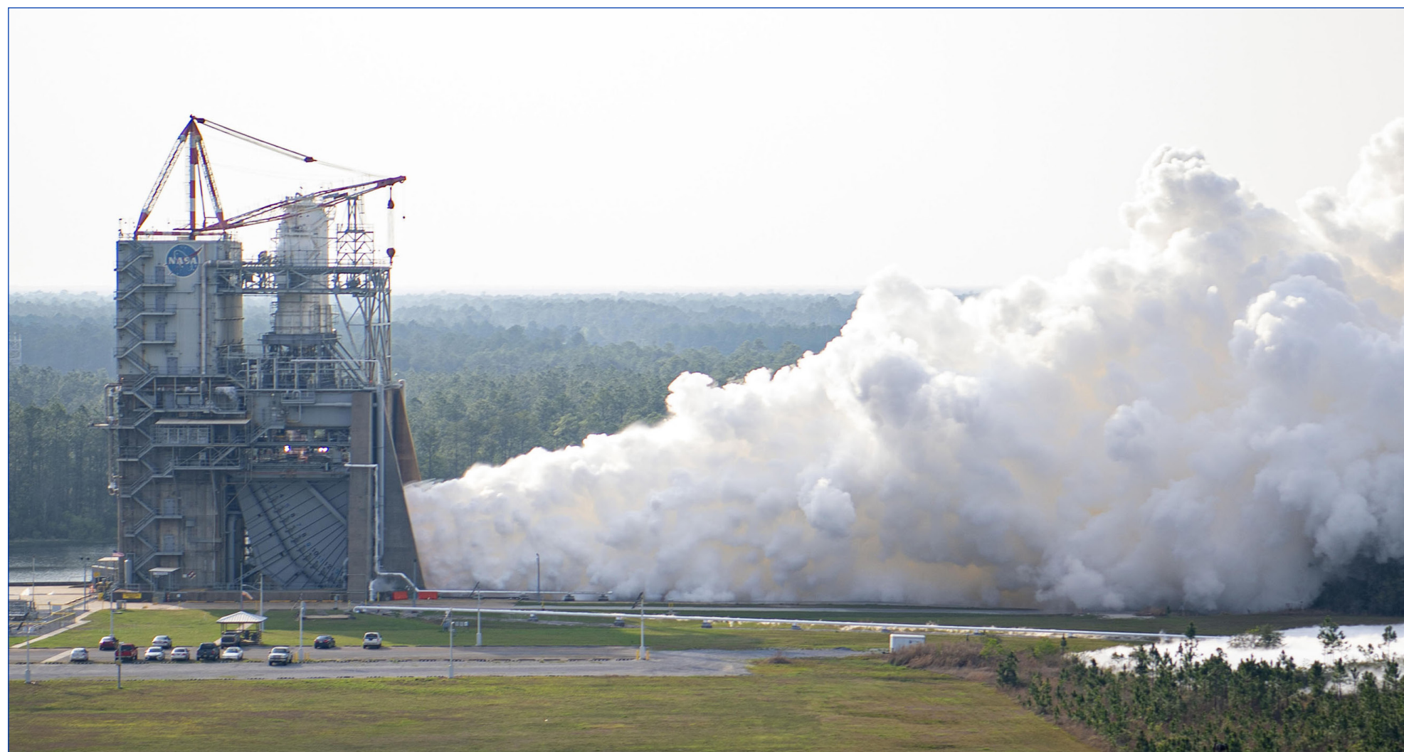
NASA conducts an RS-25 hot fire test on the Fred Haise Test Stand at NASA's Stennis Space Center in south Mississippi on March 8, 2023.
