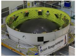
Small satellites, called CubeSats, are shown secured inside NASA's Orion stage adapter. The ring-shaped stage adapter will be connected to the Space Launch System's Interim Cryogenic Propulsion Stage, and the Orion spacecraft will be secured on top. The CubeSats will conduct a variety of science experiments and technology demonstrations that will expand our knowledge of the lunar surface during the Artemis mission. Maine's MESAT1 was selected as one of the small research satellites.
