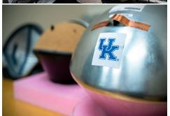
The Kentucky Re-Entry Probe Experiment (KREPE) demonstrates an affordable technology for re-entry experiments and provides flight data on Thermal Protection Systems (TPS) to help validate computational models.
