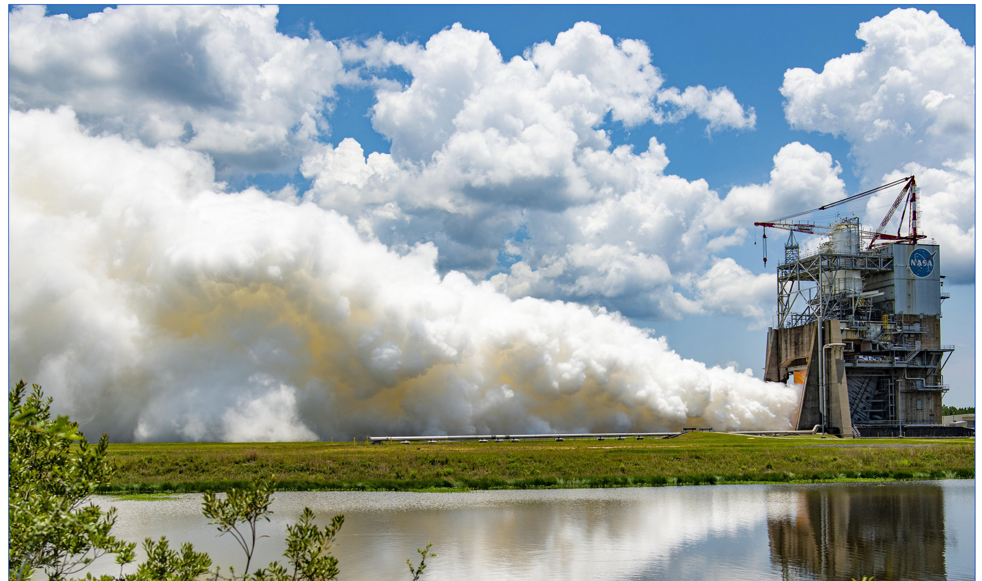
NASA conducts an RS-25 hot fire test on the Fred Haise Test Stand at NASA's Stennis Space Center on June 22. The 12-test series for the initial certification series is complete, with a second certification series to follow that will pave the way for production of new RS-25 engines to help power the SLS rocket.
