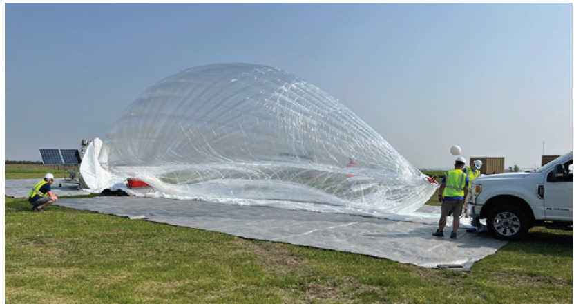
Aerostar crew inflate a high-altitude balloon in preparation for flight testing three TechLeap Autonomous Observation Challenge technologies on May 24, 2023. Credits: Aerostar
