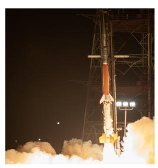
The VLF trans-lonospheric Propagation Experiment Rocket, or VIPER is studying very low frequency radio, or VLF, waves that are produced by both natural (e.g., lightning) and artificial means. During the day these waves are trapped or absorbed by the Earth's ionosphere. At night, however, some of the waves escape through the ionosphere and accelerate electrons in the Van Allen Radiation Belt. A University of Iowa insturment was involved in this NASA mission.
