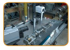
The microballistic powder gun has target heating capability and excellent impact accuracy at consistent velocities.
