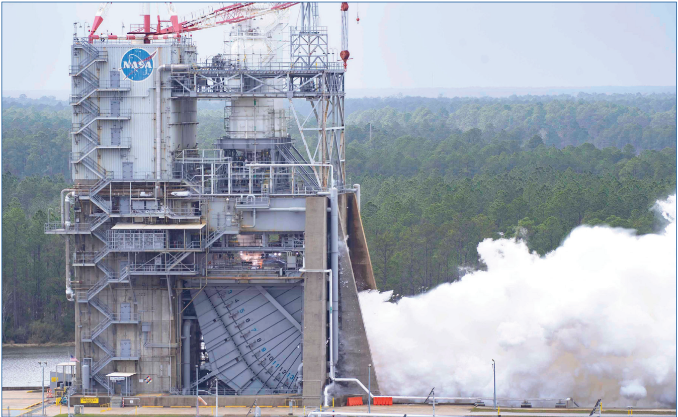
NASA conducts an RS-25 hot fire on the Fred Haise Test Stand at Stennis Space Center in south Mississippi on Feb. 8, 2023.
