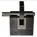
**Shear testing** is accomplished by exerting pressure (shear force) in the transverse plane of the sample until shear failure occurs.
