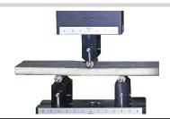
**Bend testing** is a procedure to determine the relative ductility of metal that is to be formed (usually sheet, strip, plate or wire) or to determine soundness and toughness of metal (after welding, etc.) The specimen is usually bent over a specified diameter mandrel. The four general types of bends are: free bend, guided bend (ASTM E190), semi-guided bend (ASTM E290), and wrap-around bend.
