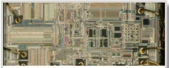
**Destructive physical analysis** is a systematic approach to disassembly of a component, electronics board, part, etc., and evaluating it down to the basic material and construction level.
