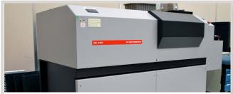
**OES testing** can absolutely verify the chemical composition of metals. This can be critical in ensuring that the correct alloy is being implemented in the design application for which it is intended.
