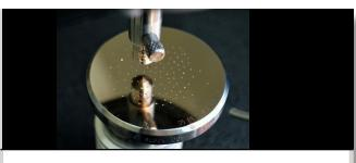
The Rockwell hardness test method consists of indenting the test material with a diamond cone or hardened steel ball indenter. The permanent increase in depth of penetration, resulting from the application and removal of the additional major load, is used to calculate the Rockwell hardness number.
