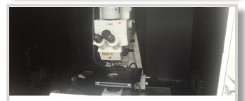
The purpose of **emission microscopy** is to detect microcircuit failure sites by light emission leakages.
