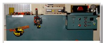
**Wire and cable testing** is performed by conducting multiple tests including spark testing, cold bend, dimensional, etc.
