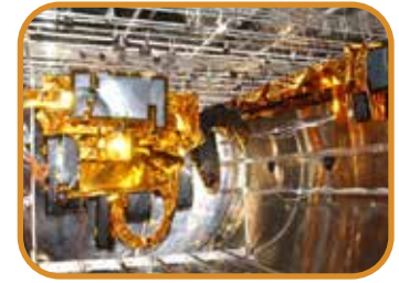
MLI Blanket Bakeout in Vacuum Chamber V7
