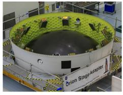
Small satellites, called CubeSats, are shown secured inside NASA's Orion stage adapter. The ring-shaped stage adapter will be connected to the Space Launch System's Interim Cryogenic Propulsion Stage, and the Orion spacecraft will be secured on top. The CubeSats will conduct a variety of science experiments and technology demonstrations that will expand our knowledge of the lunar surface during the Artemis I mission.
