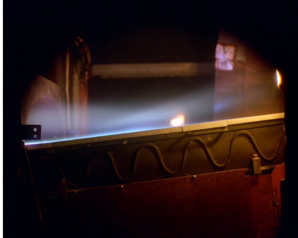
Figure 4.1.0.3. 24×24 in (61×61 cm) panel being tested in the arc jet complex
