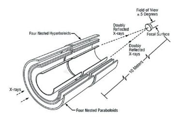
The High Resolution Mirror Assembly is contained in the cylindrical "telescope" portion of the observatory. The entire length of the telescope is covered with reflective multi-layer insulation that assists heating elements inside the unit in keeping a constant internal temperature. By maintaining a precise temperature, the mirrors within the telescope are not subjected to expansion and contraction, thus ensuring greater accuracy in observations.
