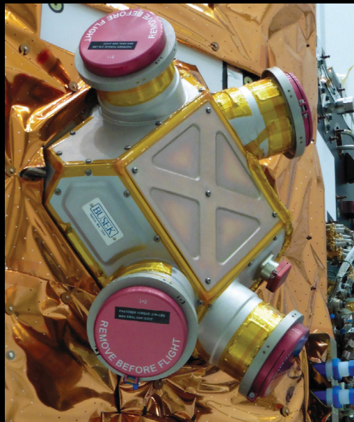
Busek cluster of four colloid microthrusters as flown on the LISA Pathfinder Mission. Source: ESA/Airbus
