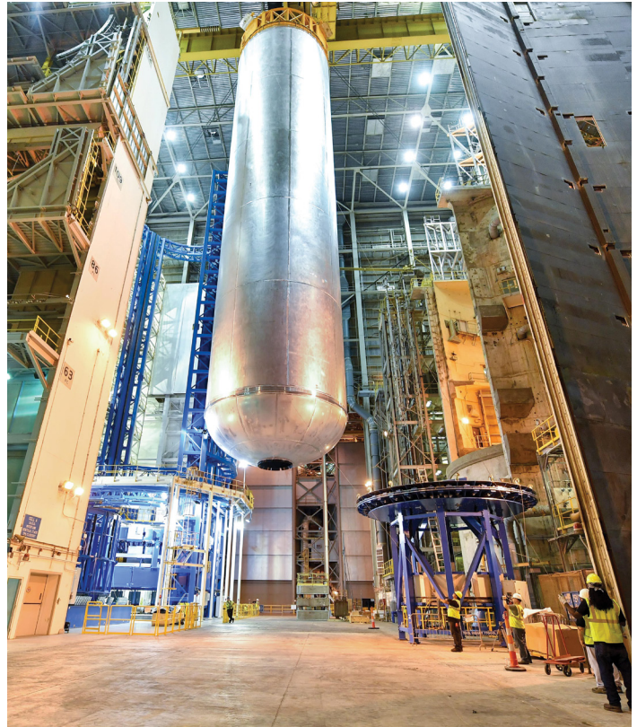
The SLS core stage Al-Li liquid hydrogen propellant tank shown after welding at NASA's Michoud Assembly Facility.
