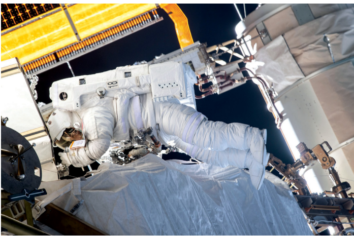
NASA astronaut Christina Koch installs Li-ion batteries in an ISS power system upgrade.
