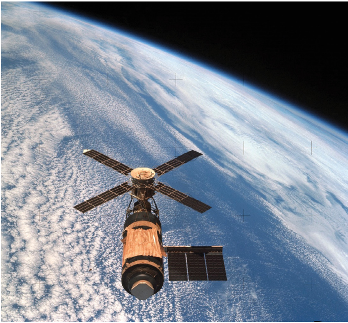
During launch of Skylab 1, there was a complete loss of the micrometeoroid shield from around the lab and damage to a solar array. Repairs made during the Skylab 2 mission included installing a sunshade for thermal control and releasing the damaged solar array.
