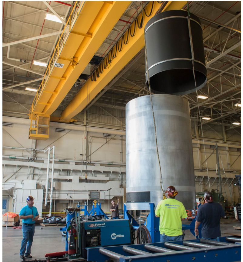
Removal of 8-ft-diameter sandwich composite test article from the tool after fabrication and before preparation for test at MSFC.
