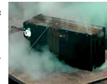
Extravehicular Mobility Unit Portable Life Support System (PLSS) Li-Ion battery redesign/testing
