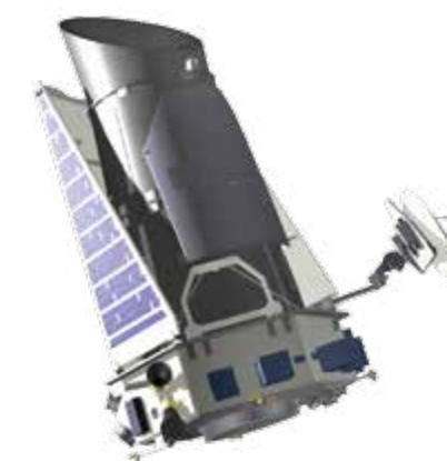
The Kepler Spacecraft relied on reaction wheels for precision pointing during its primary mission. (illustration)
