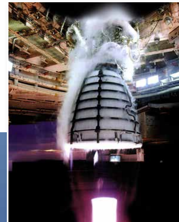
Test firing of an RS-25 engine in the A1 Test Stand at SSC.
