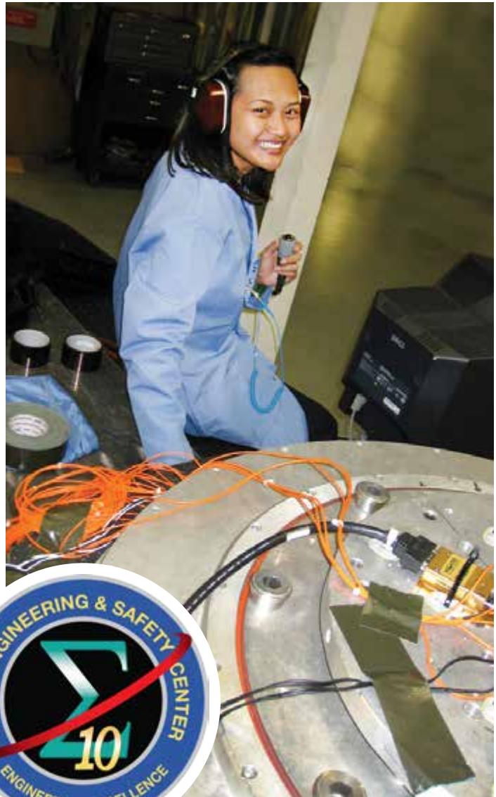
Sarah Pham conducting vibration testing of flight-test avionics.
