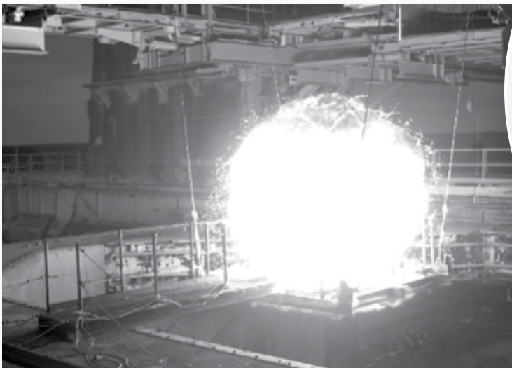
Photo: Explosion of a hydrogen-oxygen filled balloon on the B-1 Test Stand at NASA Stennis Space Center. The Hydrogen Unconfined Test Apparatus (HUCTA) device used for generating the near spherical explosion was provided by Bangham Engineering, Inc. Illustration: CFD Predictions of the HUCTA device. Grey scale contours are a numerical Schlieren image depicting shock and compression waves ahead of the flame front. The combustion zone is indicated by the superimposed color contours of gas temperature.
