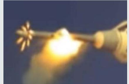
Ground test of a full-scale ACM for the LAS (left). ACM seen operating during the Pad Abort-1 flight test.
