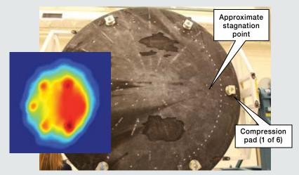
EFT-1 flown heatshield with corresponding temperature map.
