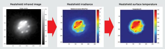
Conversion from infrared pixel counts to heatshield temperature map.
