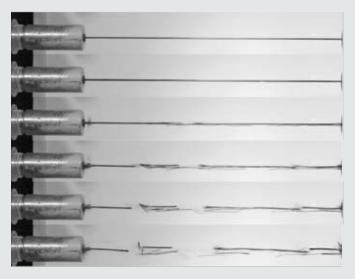
Failure of a carbon strand test specimen captured by high-speed video.
