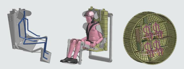
Human vibration FE model (left), anthro-pomorphic test dummy FE model (center), and representative seat placement for coupled loads analysis (right).
