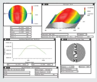
An output from the phase shifting interferometer looking through an acrylic window pane. Note the fringe pattern in the lower right and the subsequent calculated optical path length information shown in the other display boxes.
