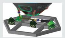
Innovative mechanism that uses low-stretch straps to route point loads to a structure.
