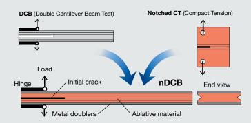
Combining the nDCB and notched compact tension tests into the new notched nDBC test.
