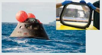
Wavefront measurements were used to characterize Orion CM window flatness
