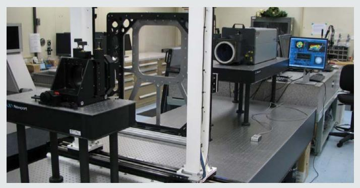
The wavefront measurement system is composed of a 6-inch aperture phase shifting interferometer on a vibration isolated optical table with a 2-D scanning system. This allows the optical path length to be measured across large spacecraft windows as well as individual panes.
