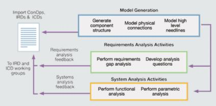
A model-based systems engineering approach was used to determine completeness of CM-ESM interfaces.
