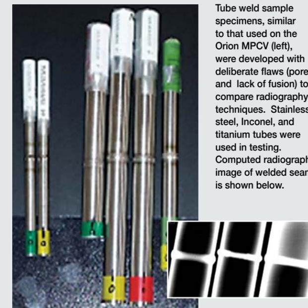
Tube weld sample specimens, similar to that used on the Orion MPCV (left), were developed with deliberate flaws (pores and lack of fusion) to compare radiography techniques. Stainless steel, Inconel, and titanium tubes were used in testing. Computed radiography image of welded seam is shown below.
