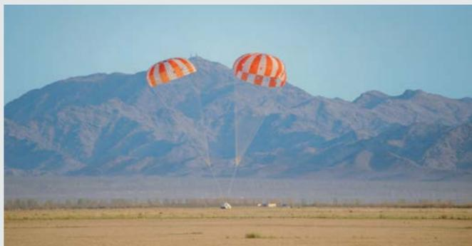
CPAS drop test of one-main-parachute-out configuration.
