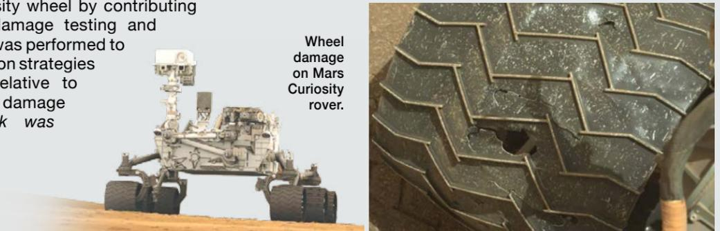
Wheel damage on Mars Curiosity rover.
