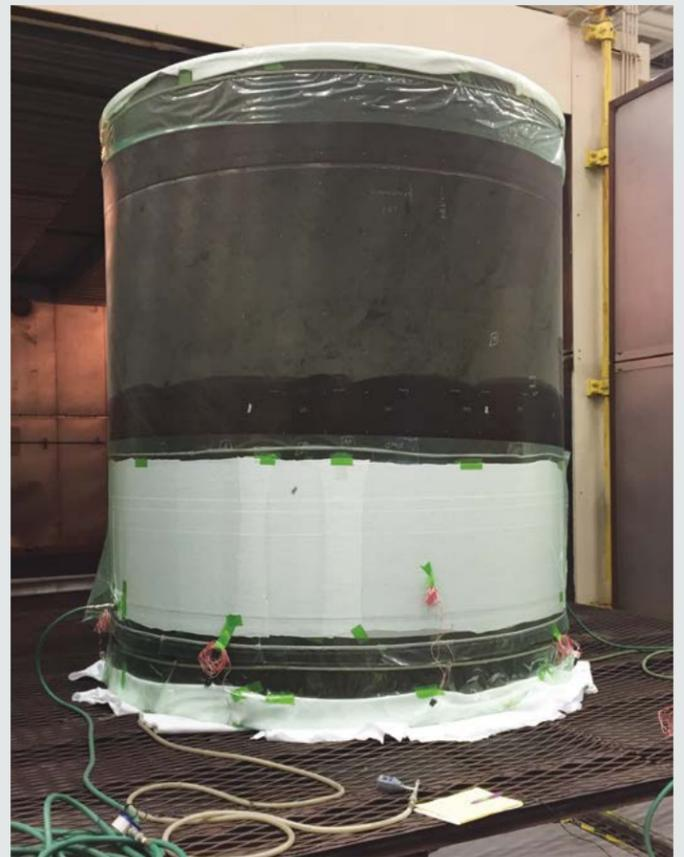
SBKF's 8-foot diameter composite shell test article.
