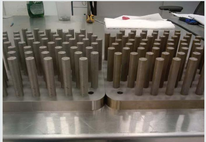
Test specimens developed by additive manufacturing with unique identifiers included on ends.
