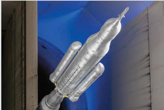
SLS model with canted ogive booster nose configuration in LaRC's Transonic Dynamics Tunnel.
