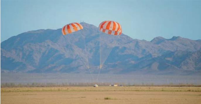
CPAS drop test of one-main-parachute-out configuration.
