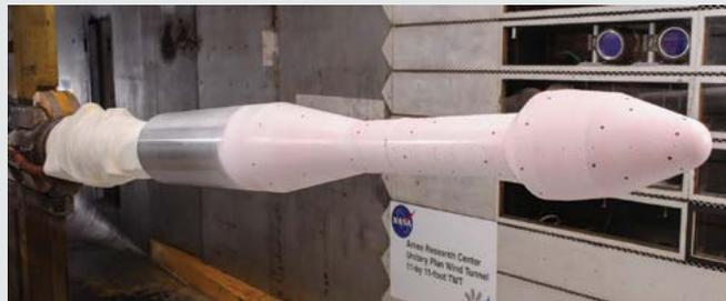
Generic launch vehicle configuration of Coe and Nute in the ARC Unitary Plan Wind Tunnel. The model is covered with pressure sensitive paint to investigate new means of measuring fluctuating pressures (see below).
