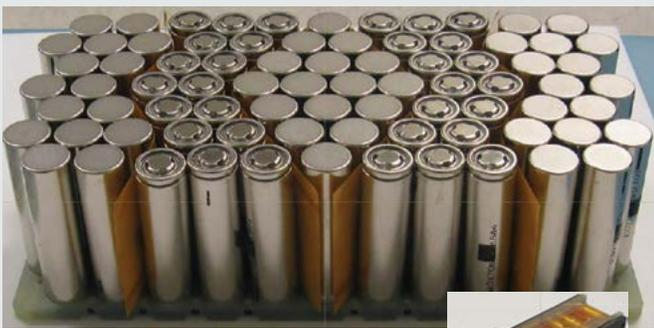
EMU batteries are composed of numerous, individual Li-ion cells, packaged in a brick fashion (inset).
