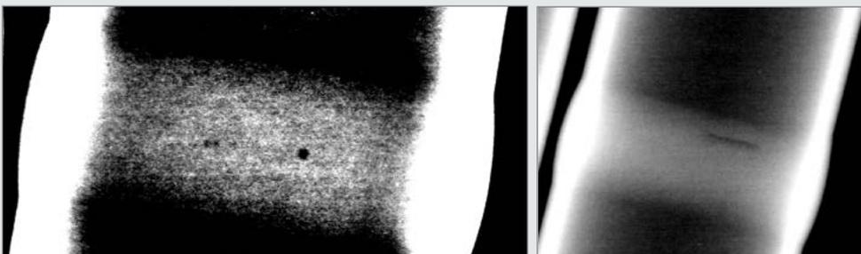
Tube weld sample specimens with small dual-pore and large single-pore defects, far left, and lack-of-fusion defects, left, were used to evaluate x-ray NDE techniques. The ability of inspectors to detect the defects using film and computed radiography were examined. Computed radiography proved to be superior to film in these tests.
