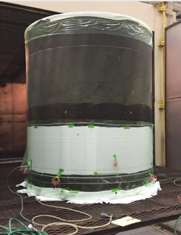
SBKF's 8-foot diameter composite shell test article.
