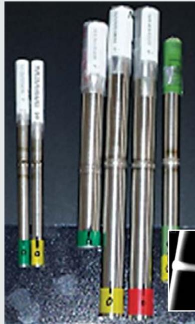
Tube weld sample specimens, similar to that used on the Orion MPCV (left), were developed with deliberate flaws (pores and lack of fusion) to compare radiography techniques. Stainless steel, Inconel, and titanium tubes were used in testing. Computed radiography image of welded seam is shown below.
