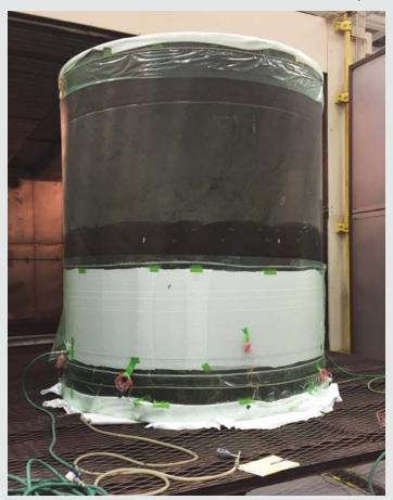
SBKF's 8-foot diameter composite shell test article.
