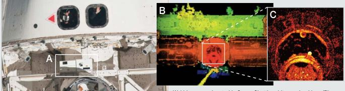
(A) Lidar sensor located in Space Shuttle orbiter payload bay. (B) Lidar-sensed intensity image of ISS docking adaptor. (C) Lidar-sensed closeup of ISS docking adaptor.
