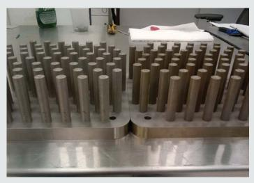
Test specimens developed by additive manufacturing with unique identifiers included on ends.
