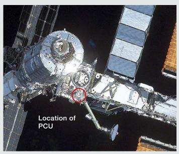
Location of the plasma contactor unit on the ISS.
