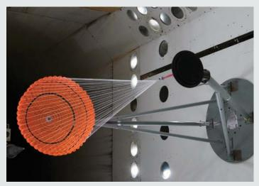
Supersonic ringsail parachute in LaRC's Transonic Dynamics Tunnel.
