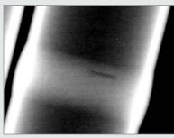
Tube weld sample specimens with small dual-pore and large single-pore defects, far left, and lack-of-fusion defects, left, were used to evaluate x-ray NDE techniques. The ability of inspectors to detect the defects using film and computed radiography were examined. Computed radiography proved to be superior to film in these tests.
