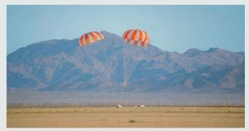
CPAS drop test of one-main-parachute-out configuration.
