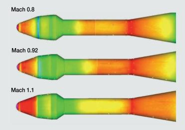
Pressure loads on the generic launch vehicle wind tunnel model were determined by time-averaged pressure sensitive paint measurements.
