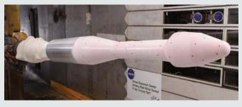
Generic launch vehicle configuration of Coe and Nute in the ARC Unitary Plan Wind Tunnel. The model is covered with pressure sensitive paint to investigate new means of measuring fluctuating pressures (see below).
