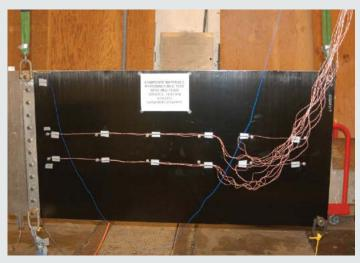
Composite panel instrumented for measurement of pyroshock loading.
