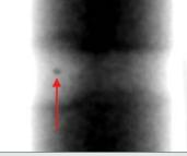
Detection of a pore in a tube weld using x-ray film, computed radiography, and digital radiography. NASA is pursuing the use of computed radiography.
