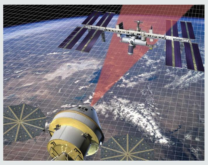
Notional representation of the Vision Navigation System flash lidar illuminating the ISS to determine range and bearing relative navigation information.
