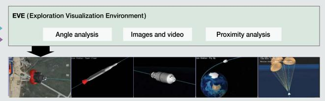
EVE combines trajectory data from POST with graphics models in a virtual environment to produce animations, proximity analysis, and angle analysis that provide insight into multi-body dynamics.
