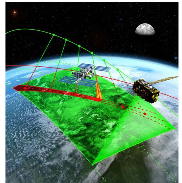
The CLARREO PFM will take measurements of Earth from the ISS with on-orbit calibration using the Sun and the Moon and improve the accuracy of other Earth-sensing instruments.
