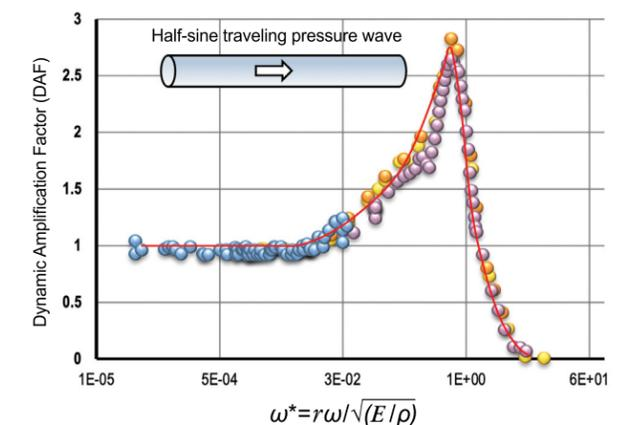
Figure 3. Design curve illustrating the effects of system characteristics on Dynamic Amplification Factor
