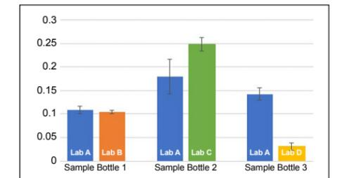
Top: Overlay of 100-ppm acetone-MEK-toluene standard (black) and ketazine HPH sample (blue) with initially unidentified contaminants identified by red arrows. Bottom: Lab-to-lab variation in initial analysis of elemental content across multiple sample bottles of HH.
