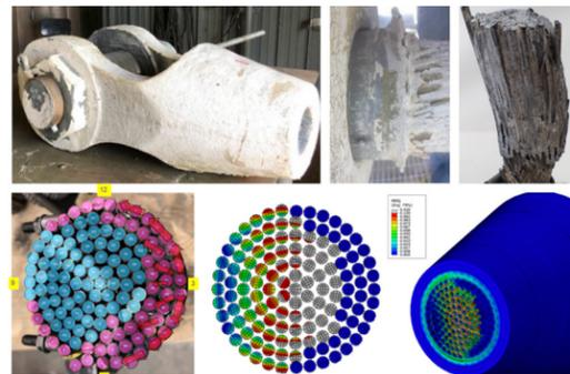
NASA Investigation of failed Arecibo Aux M4N cable/socket. Top: Socket (left); zinc extrusion (center); pulled out cable (right) Bottom: Forensic and finite element model recreation of M4N failure progression
