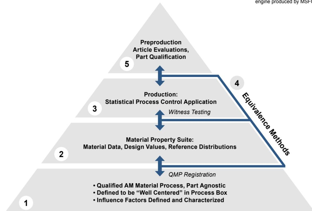
Figure 3. Material properties building block
