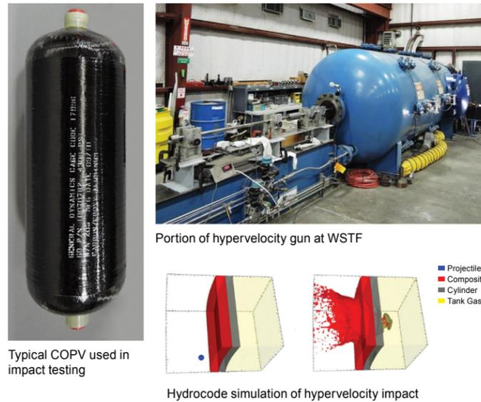
Typical COPV used in impact testing
