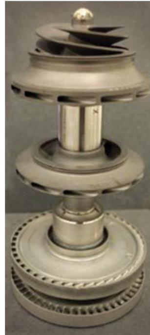
AM parts that make up the rotating assembly of the AM demonstrator engine produced by MSFC
