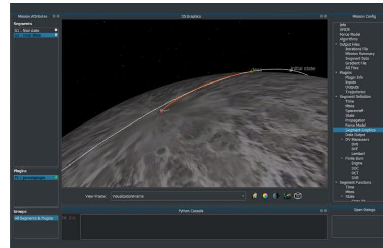
Copernicus and Genesis can be used together to enable end-to-end trajectory optimization. Here, the white trajectory is propagated by Copernicus, and the red trajectory is propagated by Genesis for a lunar descent and landing.
