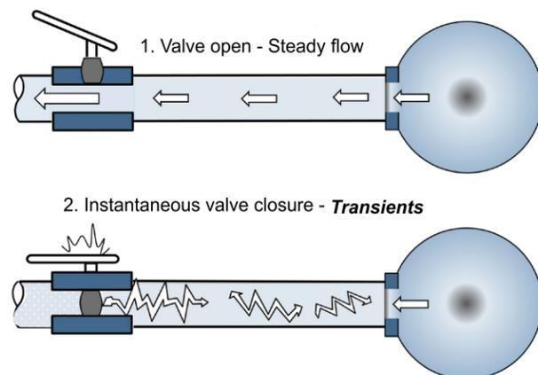
Figure 1a. Illustration of pressure transients
