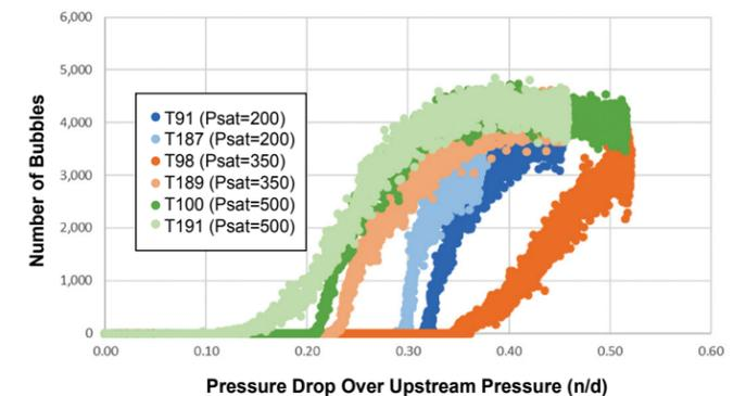
Figure 4. Total number of bubbles versus normalized pressure drop for MON-3
