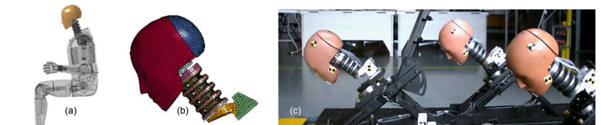
Examples of ATD FEM and test hardware used in the analysis: (a) Illustration of Hybrid III ATD, (b) LSTC ATD head-neck FEM, and (c) ATD isolated head-neck test configuration
