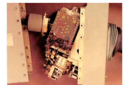
Example of flammability testing from JSC 29353B performed after the Apollo 1 fire on a vented hand controller. The fire was contained by the vented controller. Similar testing has been performed on Orion crew module components.
