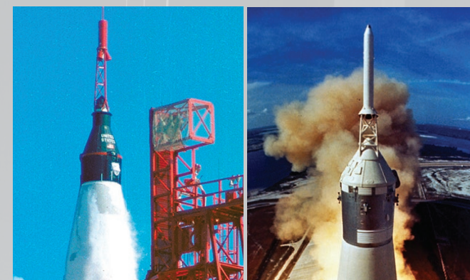
Mercury and Apollo spacecraft used launch abort towers without aerodynamically and structurally beneficial fairings.
