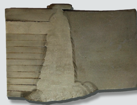
Section of weld between layered tank cylinder and single layer tank head (top) with cut-away illustration (bottom).
