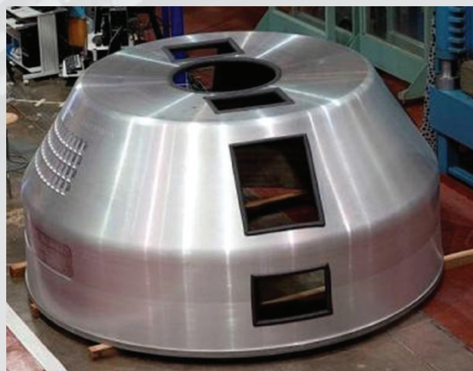
FPVBH manufactured by spin forming.
