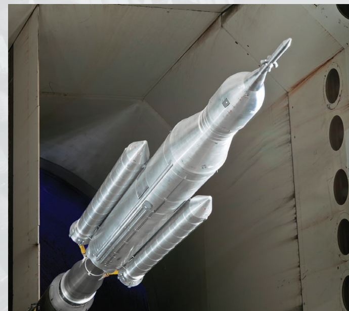
An SLS model in LaRC's Transonic Dynamics Tunnel.
