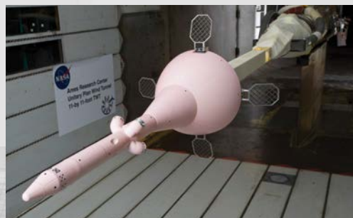
Above: ALAS fairing mounted atop a United Launch Alliance Delta IV Heavy Rocket for the EFT-1 launch. Below: After developing the ALAS shape, the NESC performed further testing in the ARC Unitary Plan Wind Tunnel to investigate stability augmentation provided by grid fins.
