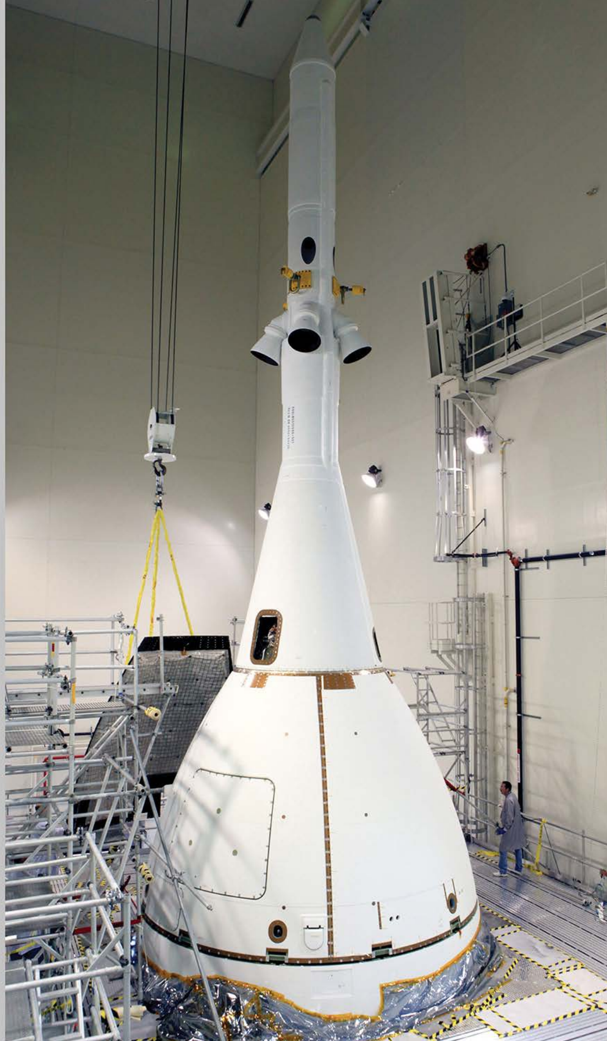
The NESC-designed Alternate Launch Abort System fairing shown integrated with the Orion spacecraft for the EFT-1 mission.
