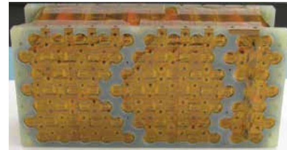
An EMU battery bank with numerous individual cells shown in holding fixture with Kapton insulation.
