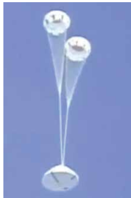
Parachute test vehicle with reefed dual drogues.
