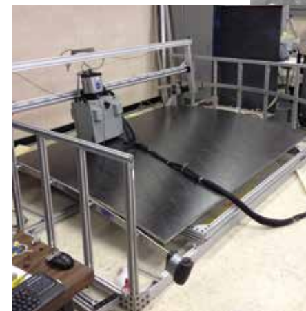
Thermal image of a defect calibration standard illustrating impact, delamination, and core separation damage types (above); LaRC Automated Thermography Scanner (left).
