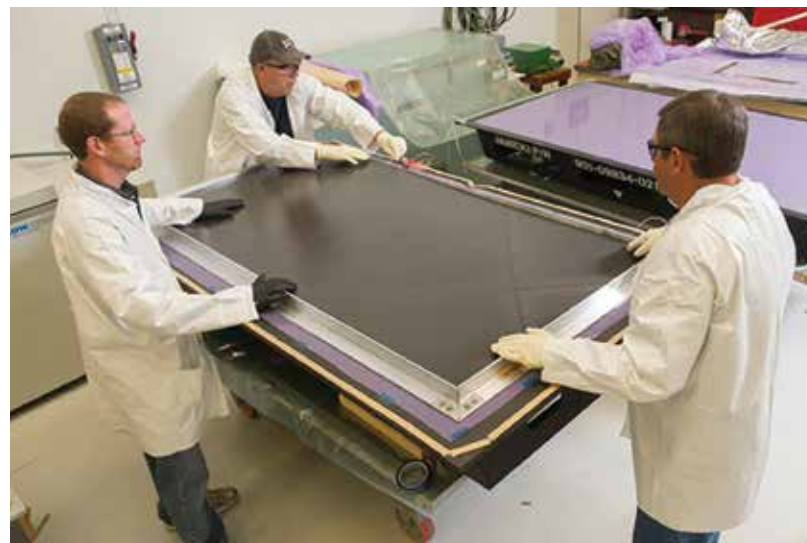
(From left) Brian Collins, James Newton, and Phillip Thompson complete fabrication of a composite panel at MSFC for pyroshock testing.
