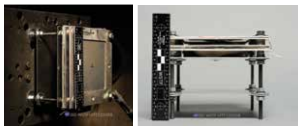
Two views are shown of a multilayered shield test target after impact from a 2.80 mm diameter aluminum particle traveling 7.38 km/s. The innermost layer of the shield was not penetrated, indicating a pass for this test.
