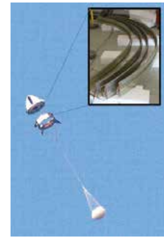
Example of frangible joint used for Max Launch Abort System.
