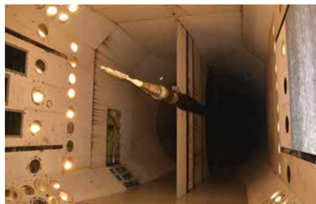
Wind tunnel shock reflection testing in LaRC's Transonic Dynamics Tunnel helped engineers evaluate the effect of shock reflections on SLS ascent performance predictions.
