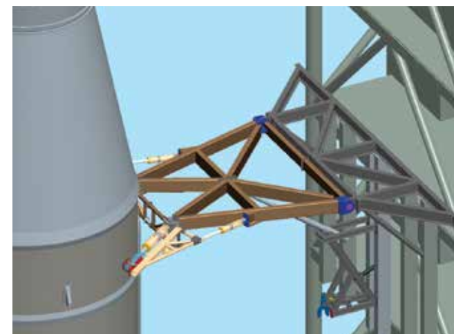
Conceptual T-0 stabilizer for SLS Block 1.
