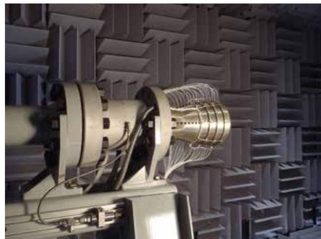
Subscale SSME testing at the University of Texas at Austin will provide data to help engineers evaluate engine startup acoustics for the SLS.
