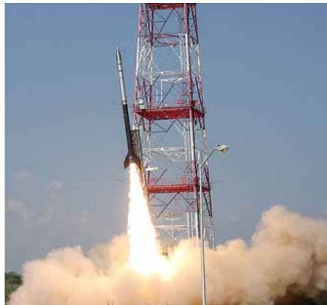
The Black Brant sounding rocket motor, operational since the 1960s, is the workhorse of NASA's Sounding Rocket Program.
