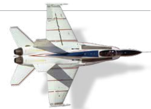
The DFRC F/A-18 is a test bed used to mature and refine the SLS adaptive control algorithm.
