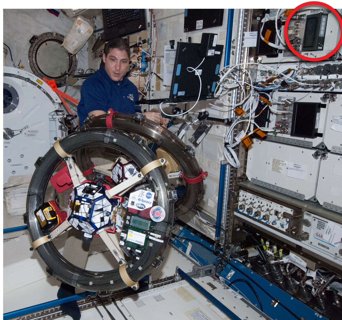
A multi-gas monitor operating in the ISS Kibo laboratory in 2014 (red circle) represents the first laser sensor to continuously measure and monitor gases on a spacecraft.
