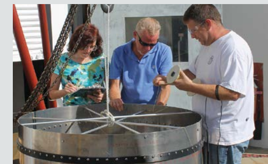
(From left) Maureen Dutton, Rick Dean, Nick Kidd of the JSC Energy Systems Test Branch examine a simulated docking mechanism jettison system tunnel section separation test firing setup.
