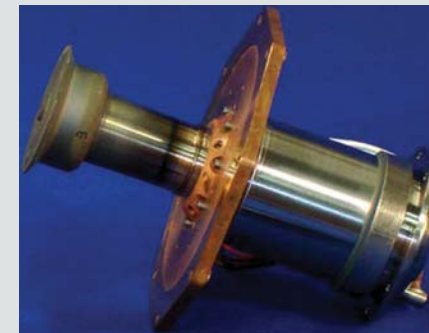
The advanced Stirling heater head is shown on the left side of the subassembly.
