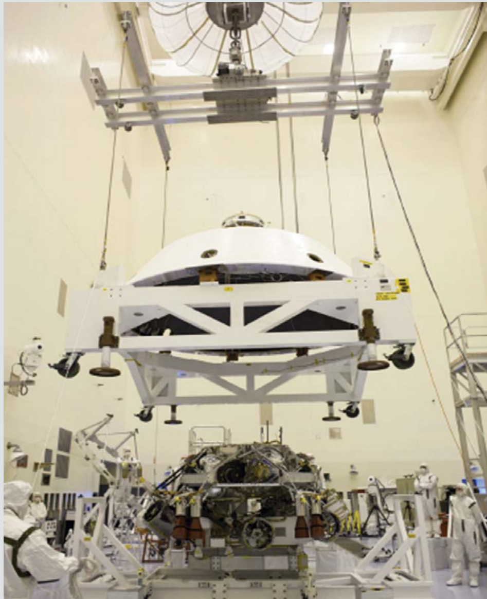
Fitting of the aeroshell to the Mars Science Laboratory rover and sky crane.
