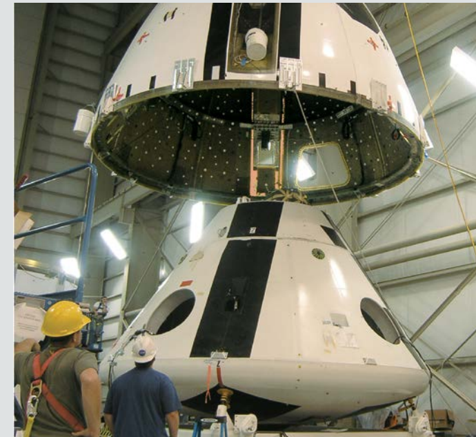
(Above) Photogrammetry was used to directly measure the CM trajectory and attitude during water impact tests at the Aberdeen Test Center, Maryland.
