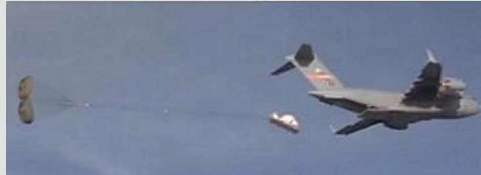
Orion boilerplate drop test article and pallet being extracted from C-17.
