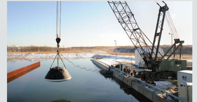
(Above) Photogrammetry was used to directly measure the CM trajectory and attitude during water impact tests at the Aberdeen Test Center, Maryland.
