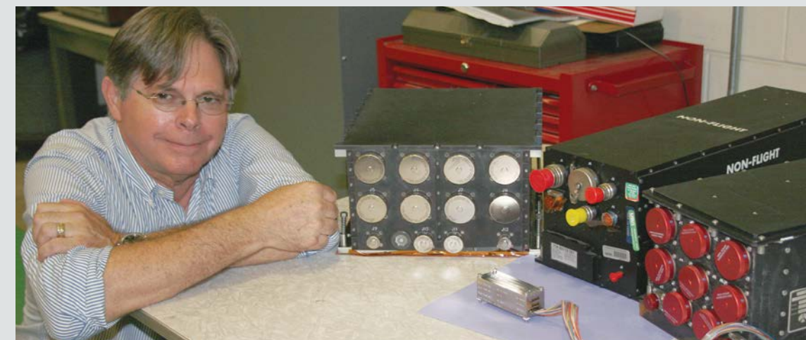
Peter Johnson compares a proposed avionics box manufactured by Quad Tron for the MLAS II flight test vehicle (foreground) with the same three shuttle-era boxes it functionally replaces.
