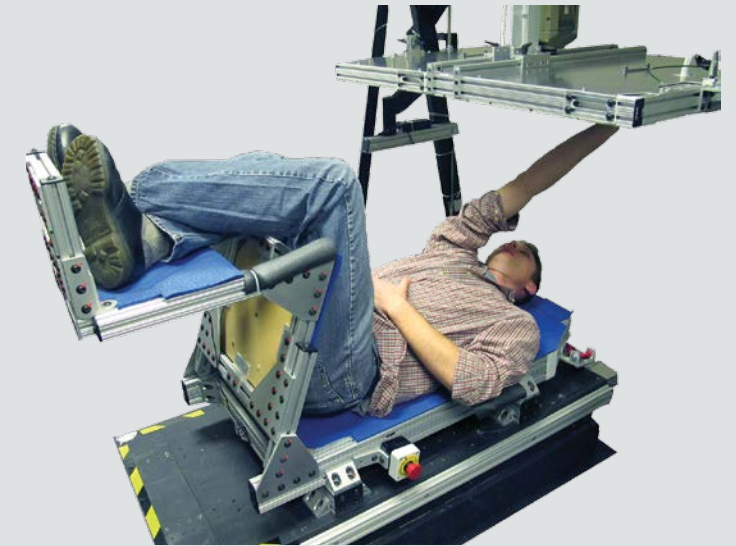
Vibration chair occupant in the ARC Human Vibration Laboratory responding via touch-screen input. Eye and head movement are recorded.
