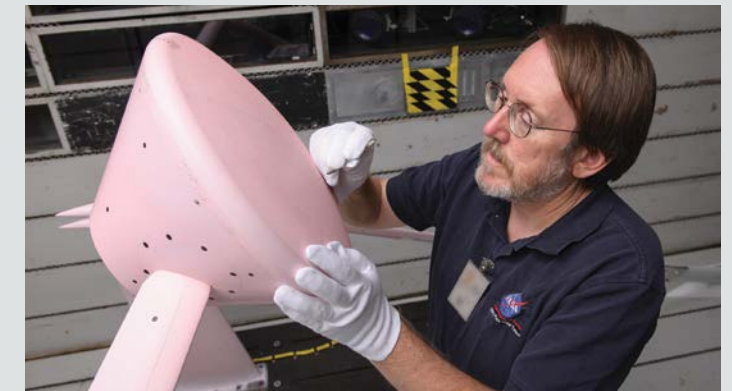
Dr. James Ross prepares a model of the Orion crew module, coated with pressure sensitive paint, in the ARC Unitary Plan Wind Tunnel.
