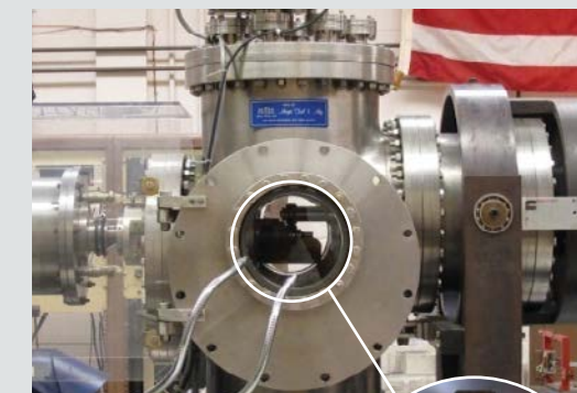
(Above) Vacuum Roller Traction Contract Rig used to characterize vacuum wear marks and debris.
