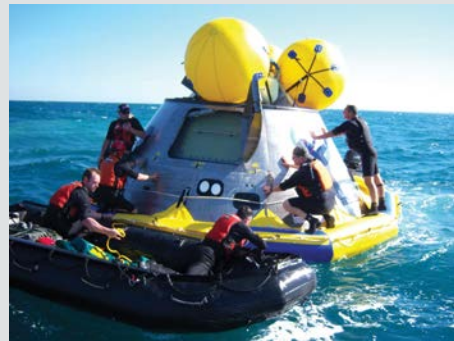
Orion MPCV recovery test article being stabilized during initial testing conducted in 2009.
