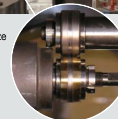
A. Rollers after 588 cycles. B. Rollers after 77,357 cycles. Rollers have a 1.5 degree misalignment.
