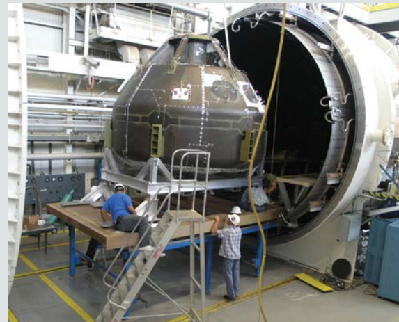
The composite crew module full-scale pressure vessel test article being readied for a vacuum test at MSFC.
