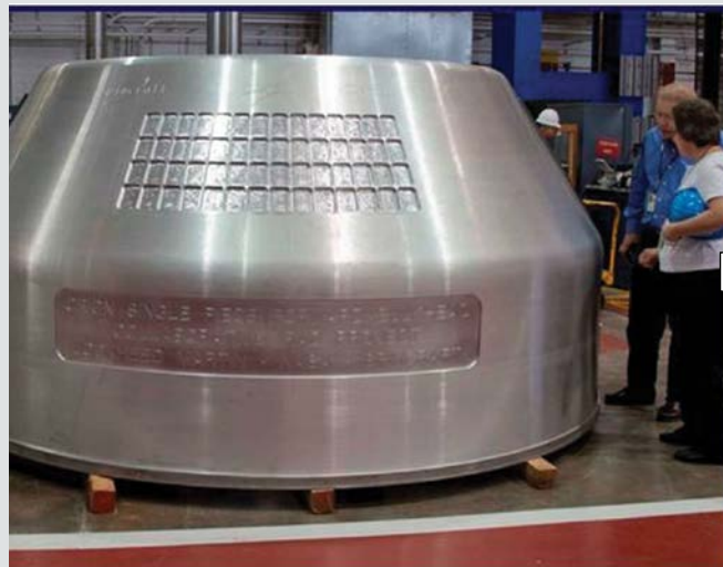
An aluminum alloy 2219 spin-formed MPCV CM-like bulkhead containing a single friction stir weld (FSW) region.
