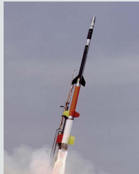
The Black Brant sounding rocket motor (black upper stage), operational since the 1960s, is the workhorse of NASA's SRP.
