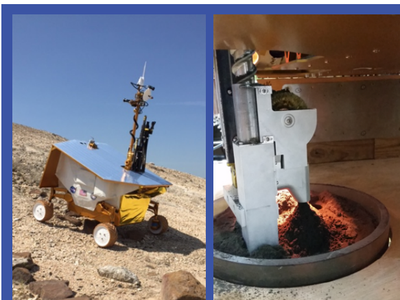
Left: In the summer of 2015, the RP prototype rover, designed and built by JSC, carried the RP payload, including NIRVSS, in rock-yard testing at JSC.
