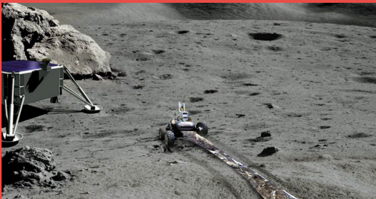
The K10 rover deploying a simulated Kapton film-based radio antenna, like that conceived for the Orion 12 Farside mission.
