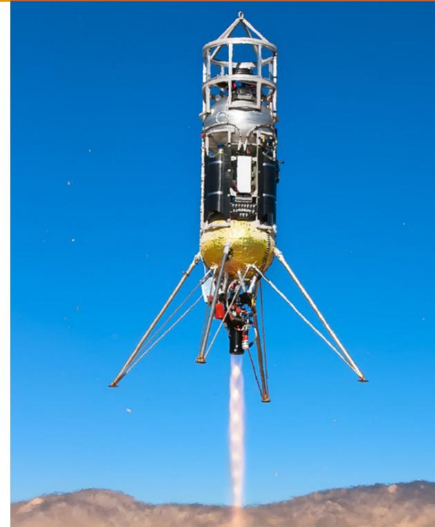
Technology for spaceflight requires testing on Earth. Masten Space Systems built Xodiac to test terrain-relative navigation and hazard-avoidance systems for landings on Mars, the Moon, and more. *Credit: Masten*
