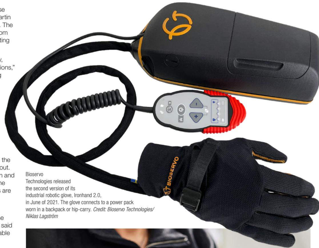
Bioservo Technologies released the second version of its industrial robotic glove, Ironhand 2.0, in June of 2021. The glove connects to a power pack worn in a backpack or hip-carry. *Credit: Bioservo Technologies/Niklas Lagström*
