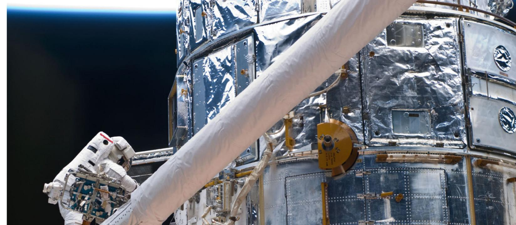
In May 2009, astronaut John Grunsfeld works on repairs to the Hubble Space Telescope, including replacing three thermal blankets protecting the telescope's electronics. This multi-layer reflective thin-film insulation, also known as radiant barrier, manages temperatures in almost all NASA spacecraft and spacesuits and is also one of the agency's most ubiquitous spinoffs, appearing in countless products, including new lightweight jackets from 13-One. Credit: NASA
