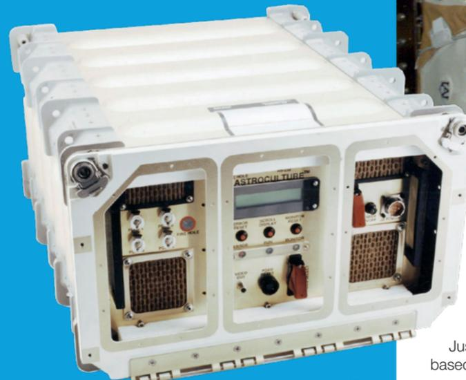
As engineers at the NASA-funded Wisconsin Center for Space Automation and Robotics built the Astroculture plant-growth chamber in the 1990s, they came up with photocatalytic oxidation as a way to prevent the buildup of ethylene, a plant growth hormone that accelerates ripening and withering. Credit: NASA
