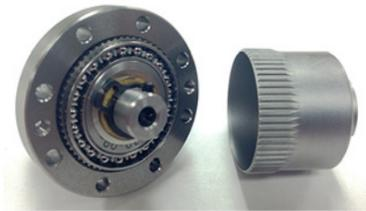
Flexsplines represent a potentially major industrial application for bulk metallic glass. The thin, flexible, cup-shaped gears are integral to the strain wave gears common in robotics. They're typically cut, ground, and drilled from steel billets in a process that is long and costly. The flexspline shown on the right, however, was injection molded from metallic glass in a cheaper, simpler process. *Credit: NASA*
