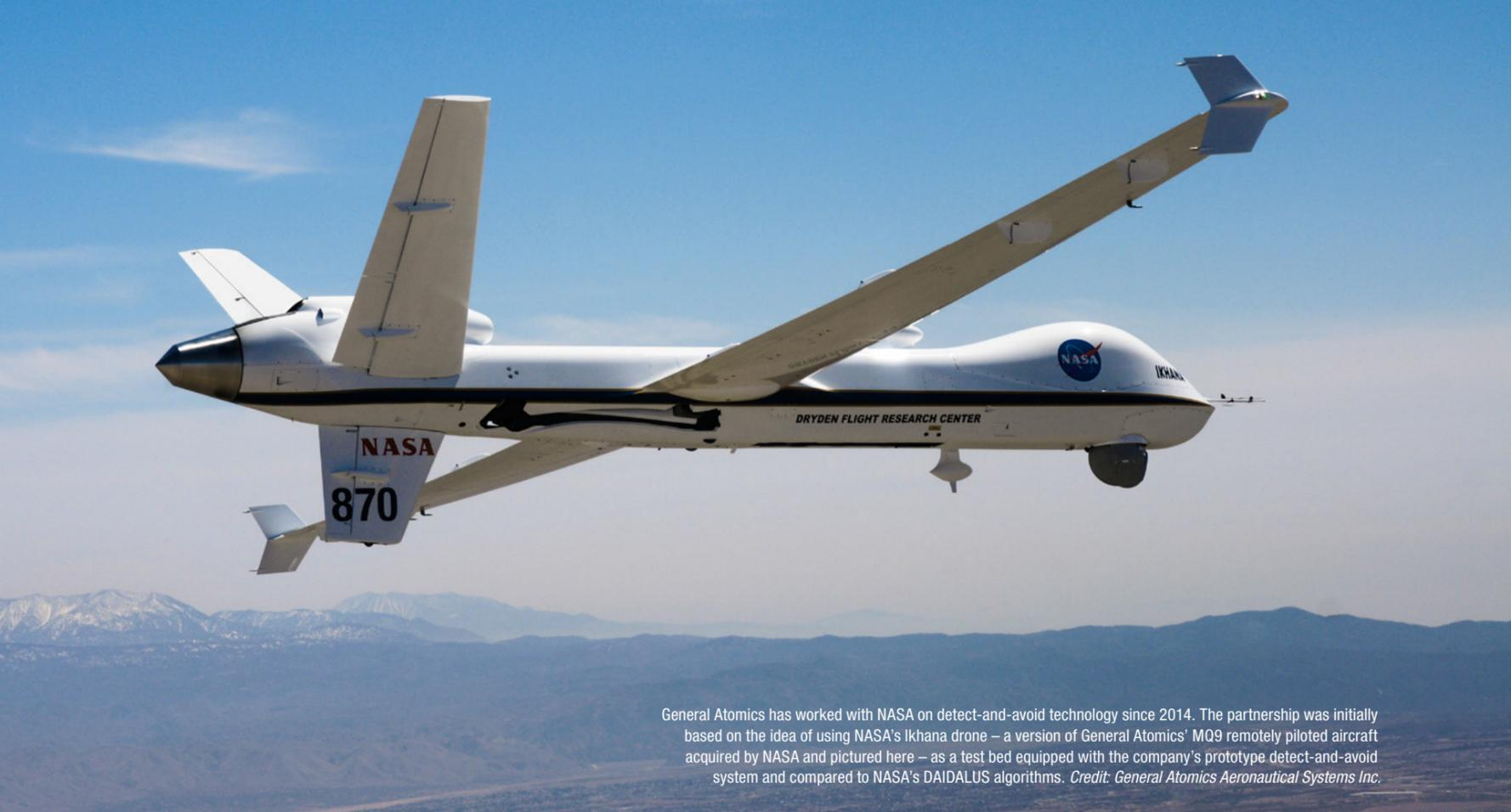
General Atomics has worked with NASA on detect-and-avoid technology since 2014. The partnership was initially based on the idea of using NASA's Ikhana drone – a version of General Atomics' MQ9 remotely piloted aircraft acquired by NASA and pictured here – as a test bed equipped with the company's prototype detect-and-avoid system and compared to NASA's DAIDALUS algorithms. *Credit: General Atomics Aeronautical Systems Inc.*
