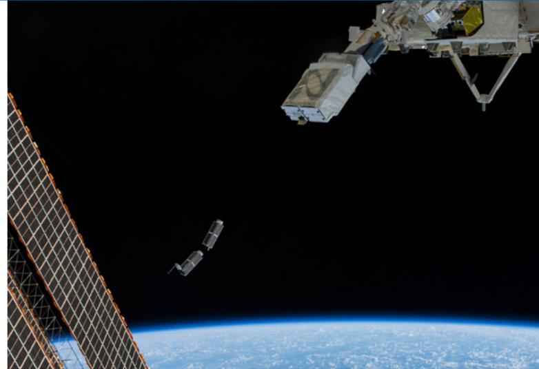
CubeSats can be used for a variety of tasks, from Earth observation to flying science experiments, but their small size makes it a challenge to assemble all the parts as well as shielding needed to manage the extreme temperatures of space. NASA is interested in new manufacturing techniques that enable more efficient use of materials. *Credits: NASA*
