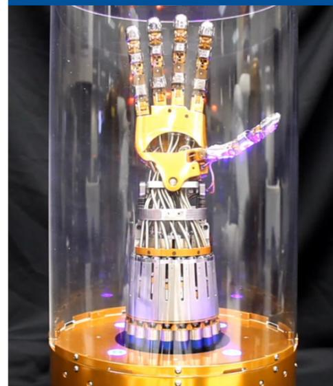
After building the hands for Robonaut 2, both NASA and GM saw potential uses for a robotic glove based on the same hardware. While the automobile manufacturer saw the potential to reduce repetitive stress injuries on factory floors, the space agency's astronauts have always had difficulty using pressurized gloves in space for extended periods. *Credit: NASA*
