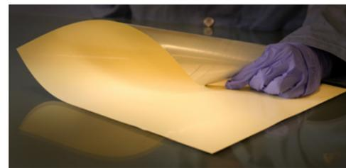
AeroZero, an ultra-thin polymer aerogel created by Blueshift Materials, laminates onto other surfaces such as the aluminum shown here. This process makes it possible to improve thermal management without adding weight or bulk. *Credit: Blueshift Materials Inc.*
