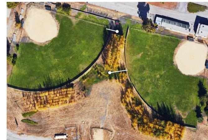
The first grove of inoculated poplars and uninoculated control trees was planted between two baseball fields at Ames. As the trees took root, center personnel installed a test well at each end of the plot to compare contaminant levels in groundwater flowing into the grove against water coming out. The results were so dramatic that the center purchased two more stands of inoculated poplars, seen here just south of each baseball field. Credit: Google Earth
