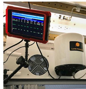
Ahead of future lunar missions, NASA wanted a sensor to act like a canary in a coal mine, warning inhabitants if the level of dust gets dangerous. Lunar Outpost developed the Space Canary, an air-quality sensor, shown here in a lunar habitat prototype designed by Lockheed Martin. Credit: Lockheed Martin Corporation
