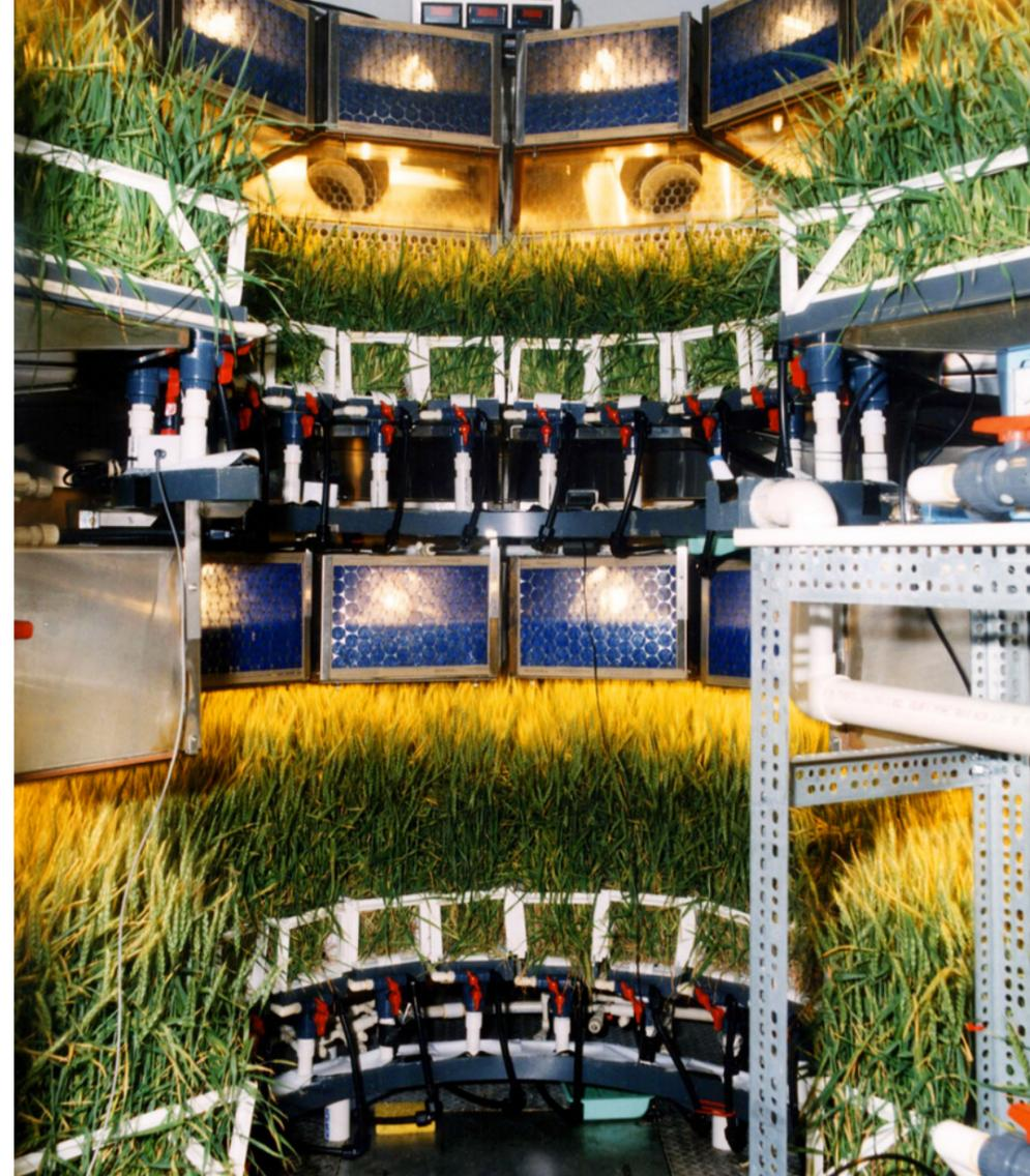
The interior of the Biomass Production Chamber at Kennedy Space Center in Florida replicated the closed growing environment astronauts will use in space or on other planets to grow fresh crops. The chamber helped NASA provide critical data for the indoor farming industry. *Credit: NASA*
