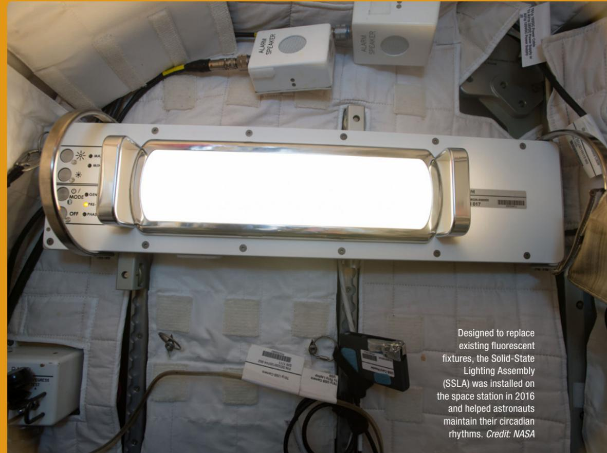
Designed to replace existing fluorescent fixtures, the Solid-State Lighting Assembly (SSLA) was installed on the space station in 2016 and helped astronauts maintain their circadian rhythms. *Credit: NASA*
