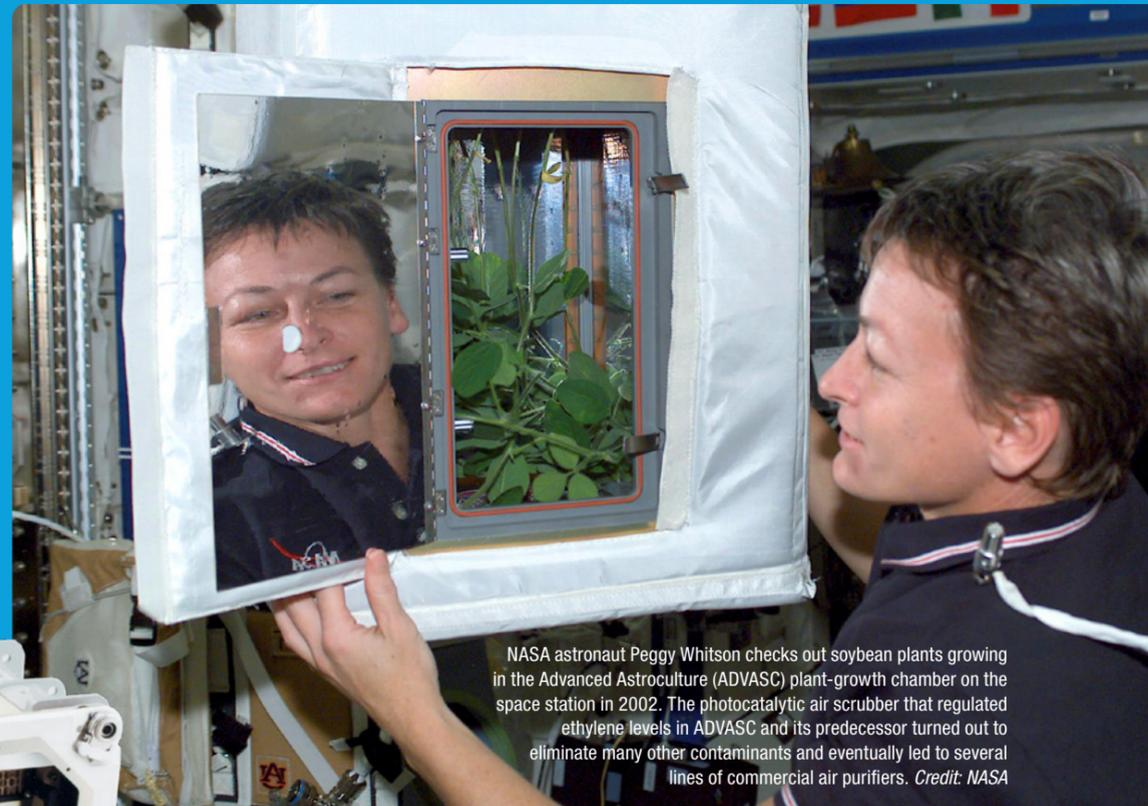
NASA astronaut Peggy Whitson checks out soybean plants growing in the Advanced Astroculture (ADVASC) plant-growth chamber on the space station in 2002. The photocatalytic air scrubber that regulated ethylene levels in ADVASC and its predecessor turned out to eliminate many other contaminants and eventually led to several lines of commercial air purifiers. Credit: NASA
