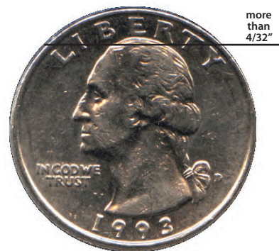
Fig. 7 Quarter (head) tread measurement
