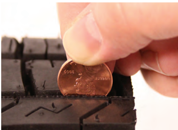
Fig. 6 Penny (head) tread measurement
