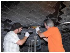
The silica tile material is referred to as LI-900. It insulates heat so well that tiles can be held bare-handed on one side even while the opposite side is still red hot. Educators can demonstrate that ability in the classroom, substituting a blowtorch for the reentry-generated heating.
