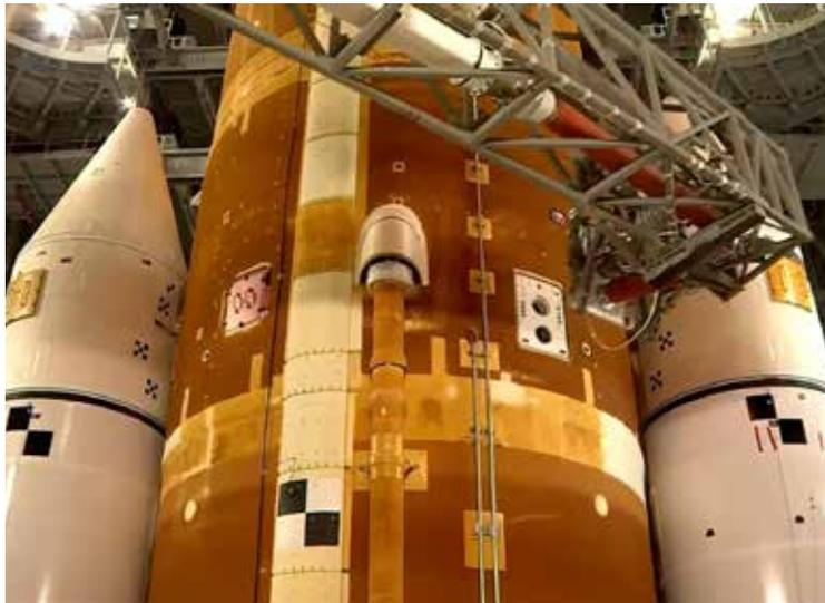
Teams at Kennedy conducted the Umbilical Release and Retract Test in September. The test ensured that the umbilicals, which supply the rocket with fuel, oxidizer, power, and commands while on the launch pad, properly separate during launch.
