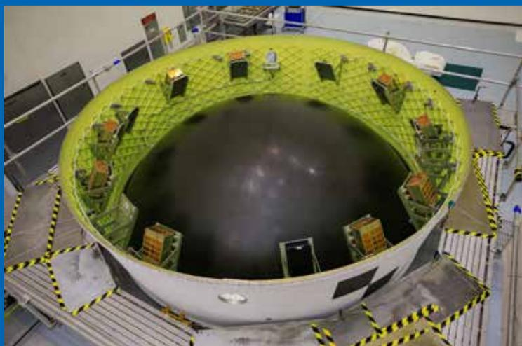
Artemis I will have 10 "hitchhiking" payloads that will deploy at various deep space destinations following Orion's separation from SLS. These briefcase-size secondary payloads will launch in the Orion stage adapter and will conduct a variety of studies around Earth, the Moon, and deeper in space. They were successfully integrated into the adapter in the fall and subsequently stacked on SLS.
