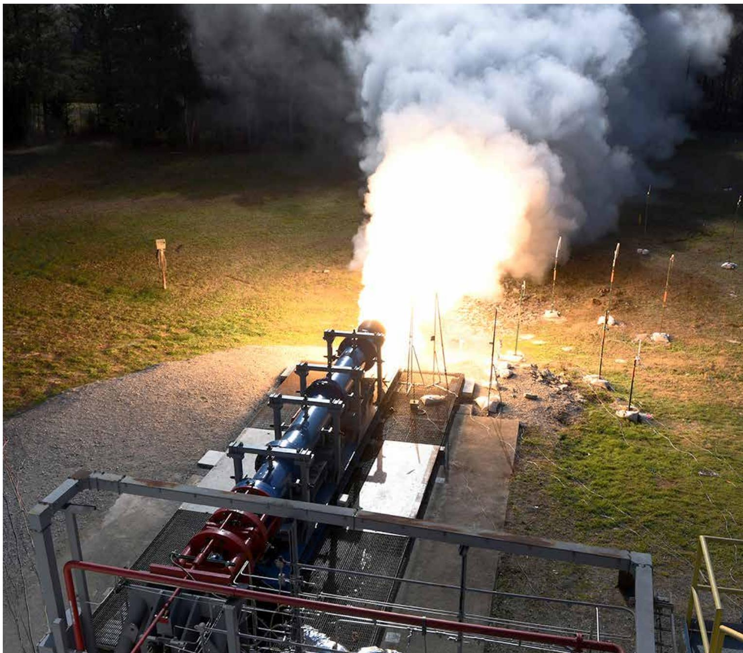
The subscale motor produced 76,400 lbs. (34,654 kg) of thrust during the hot fire test. This test was the first of two tests supporting the advanced booster development effort that includes a new motor design for upcoming Artemis missions after Artemis VIII.
