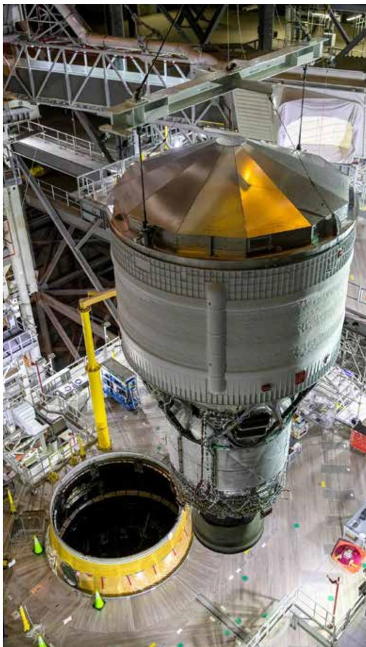
The Artemis I SLS interim cryogenic propulsion stage (ICPS) is stacked onto the launch vehicle stage adapter (LVSA).
