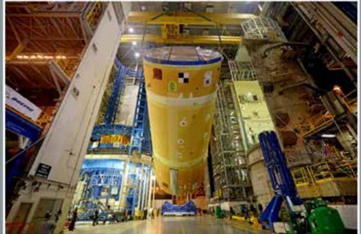
Teams at NASA's Michoud Assembly Facility in New Orleans completed joining the upper part of the core stage that will send the Artemis II crew on their lunar mission. The 66-foot-tall portion of the 212-foot-tall rocket stage consists of the forward skirt, the liquid oxygen tank, and the intertank.
