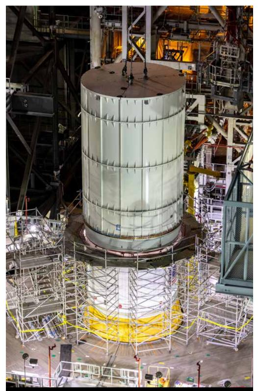
The Artemis I SLS, stacked with the Orion mass simulator and OSA structural test article, undergoes modal testing.
