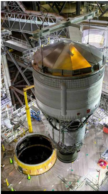
The Artemis I SLS interim cryogenic propulsion stage (ICPS) is stacked onto the launch vehicle stage adapter (LVSA).
