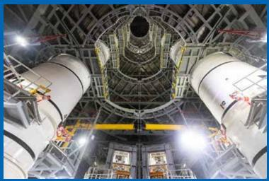
In March, the solid rocket boosters completed stacking on the mobile launcher in the Vehicle Assembly Building's High Bay 3. Stacking began in November 2020 and involved putting each of the booster segments on the mobile launcher. Following stacking, teams conducted push-pull tests to collect data on the boosters. The core stage was mated to them in the summer.
