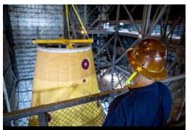
The LVSA for the Artemis I SLS is moved into position on the core stage at the Vehicle Assembly Building (VAB).
