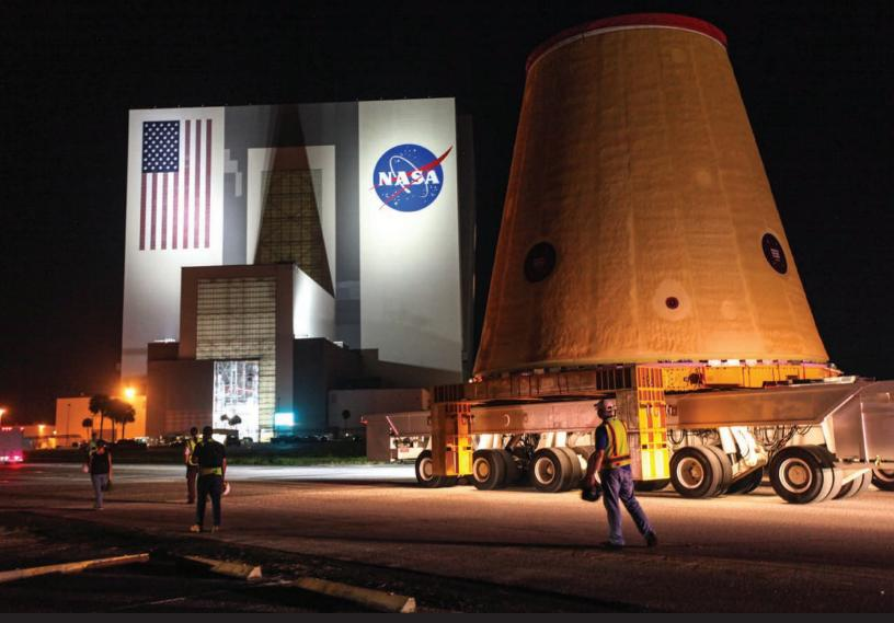
The launch vehicle stage adapter (LVSA), which connects the core stage and upper stage, shipped on NASA's Pegasus barge from Marshall Space Flight Center in Huntsville, where it was manufactured, to Kennedy Space Center in July 2020.
