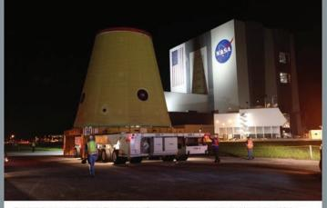
Technicians with NASA's Exploration Ground Systems moves the launch vehicle stage adapter [LVSA] for the SLS rocket to the Vehicle Assembly Building (VAB) at Kennedy Space Center July 30 for processing. The LVSA connects the SLS core stage to the rocket's upper stage and will remain in the VAB until it's time for stacking on the mobile launcher ahead of the Artemis I launch.
