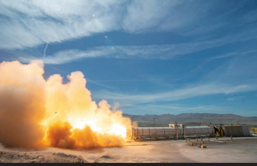
NASA and Northrop Grumman successfully completed the Flight Support Booster-1 (FSB-1) test in Promontory, Utah, Sept. 2. The NASA and Northrop Grumman team will use data from the test to evaluate the motor's performance using potential new materials and processes for Artemis missions beyond the Moon landing in 2024.
