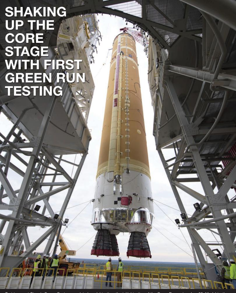
Test teams at Stennis Space Center completed modal testing, the initial testing of the Green Run series, Jan. 30. Modal testing mimics the stresses the core stage will endure during launch and verifies flight control parameters.
