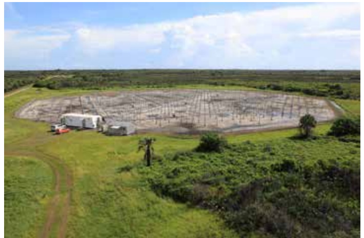
A total of 640 antennas on the five-acre site can collect wind speed and direction data from 6,000 to 62,000 feet every five minutes.
