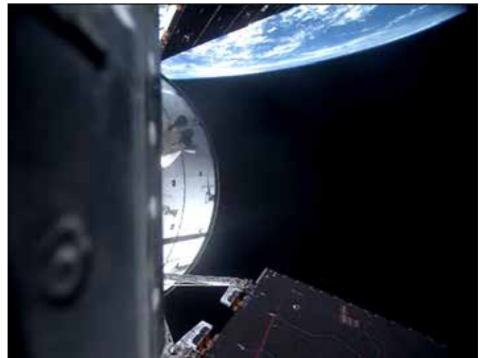
A camera on the Artemis II Orion spacecraft captured this view of the SLS (Space Launch System) rocket's interim cryogenic propulsion stage (ICPS) below the Orion and two of its solar array wings on the first day of the mission.
