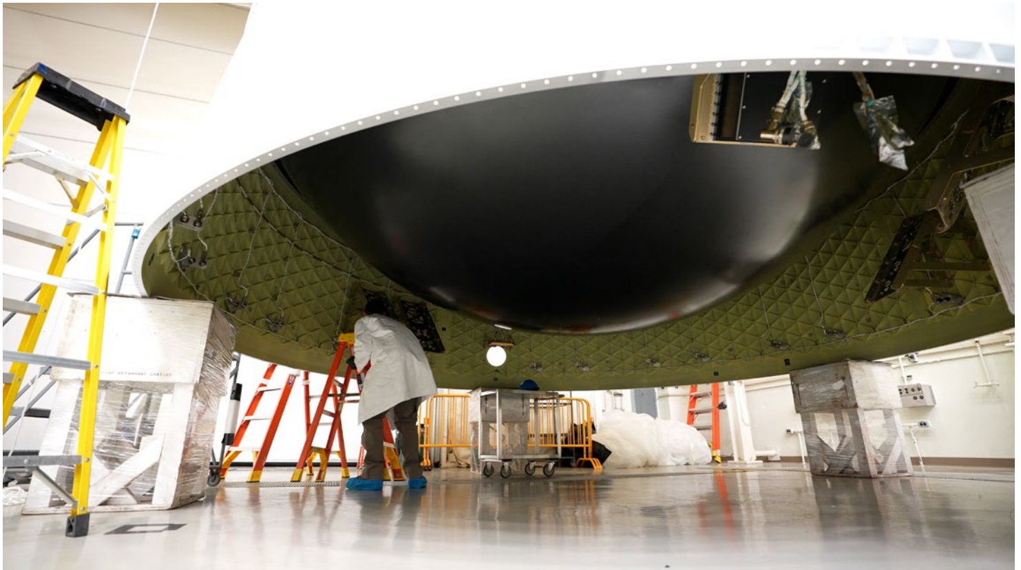
Technicians at NASA's Marshall Space Flight Center in Huntsville, Alabama, install the diaphragm of the Artemis II OSA.
