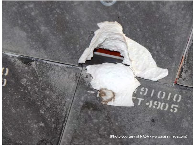
Img. 4 A damaged tile from Space Shuttle Endeavor. The tile was damaged on Mission STS-118 when a piece of foam from the external tank broke off during launch.
