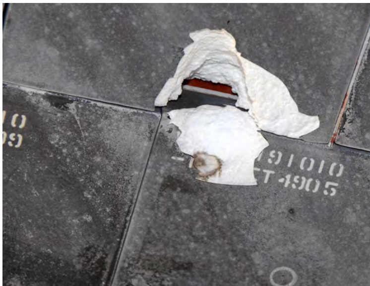
Img. 4 A damaged tile from Space Shuttle Endeavor. The tile was damaged on Mission STS-118 when a piece of foam from the external tank broke off during launch.
