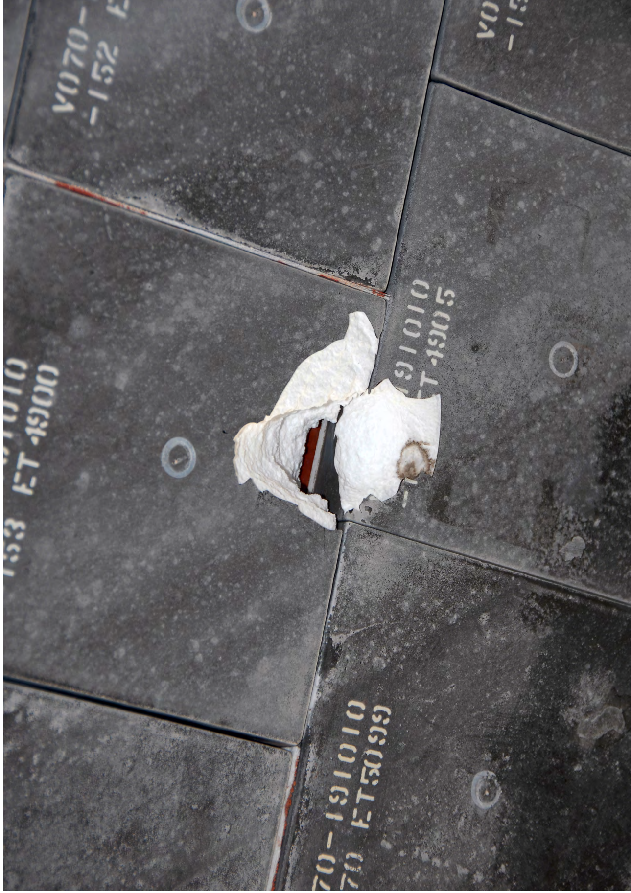
Img. 4 Shuttle tile showing signs of damage.
