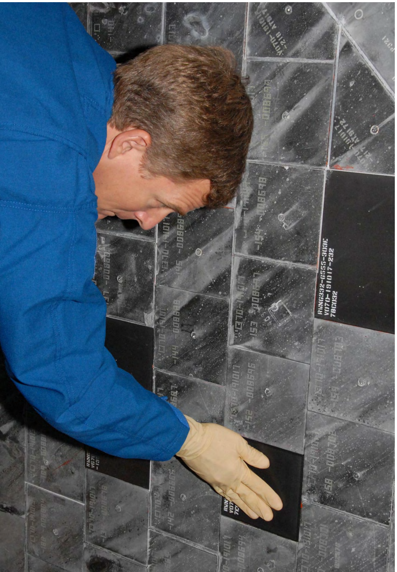
Img. 3 Replacing a shuttle tile.
