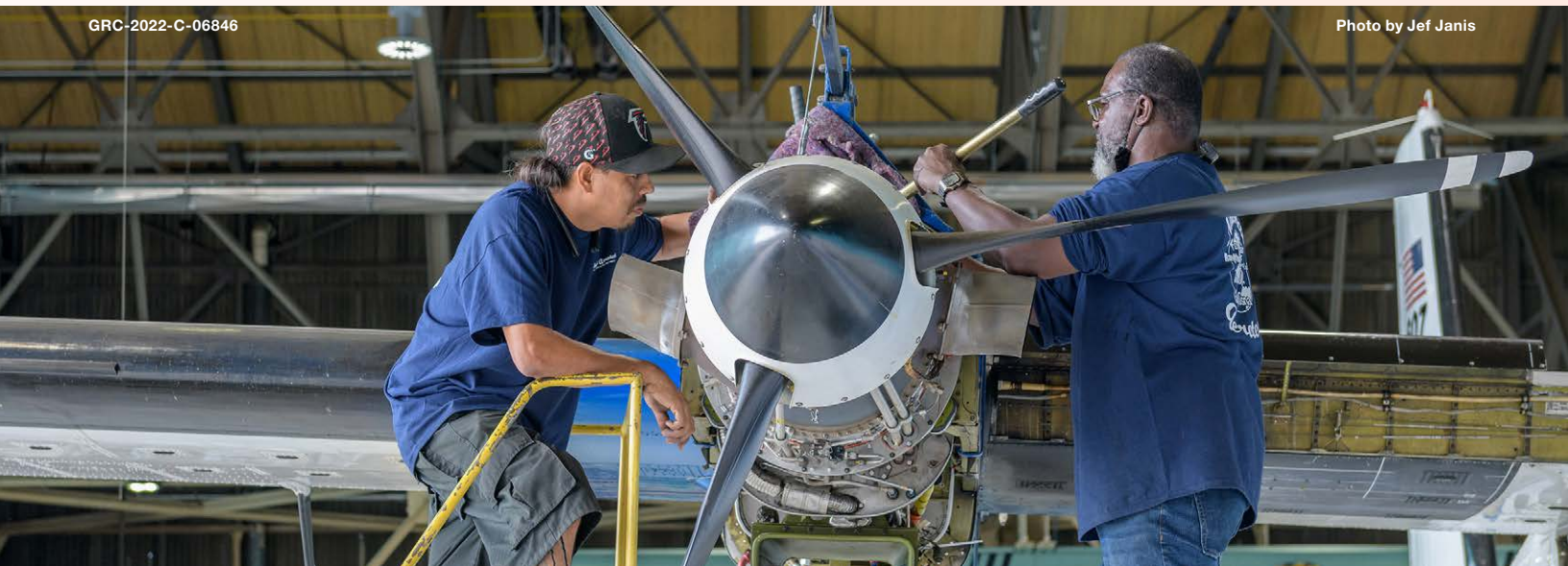
National Aerotech technicians Jaime Lujano, left, and Carl Dalrymple prepare to remove one of the DHC-6 Twin Otter's engines before its trip to MTSU.
