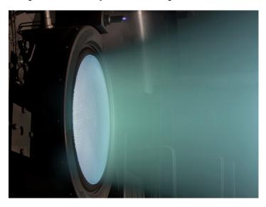
NASA's Evolutionary Xenon Thruster (NEXT) is a 7-kW, state-of-theart gridded ion thruster capable of exhaust speeds over 90,000 mph and can be operated continuously for several years, making it an attractive, enabling propulsion system for NASA deep-space science missions.
